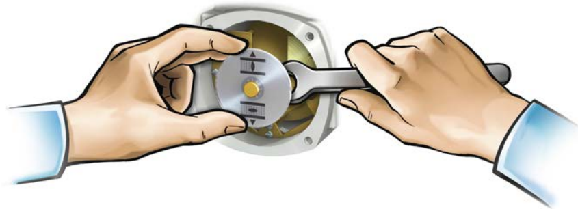
Figure 28: Pull off indicator disc
