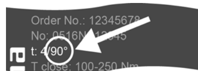
Figure 23: Example of swing angle on name plate
