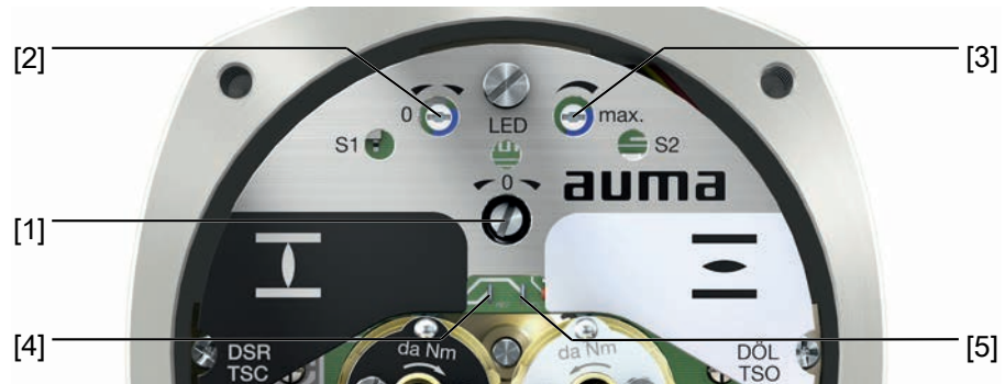
Figure 36: View on control unit when switch compartment is open
