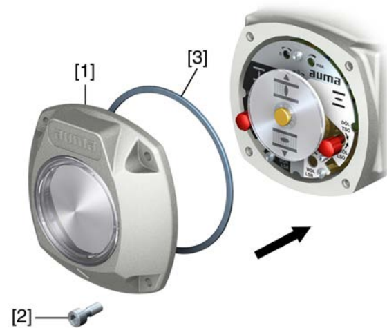
Figure 34: Close switch compartment
