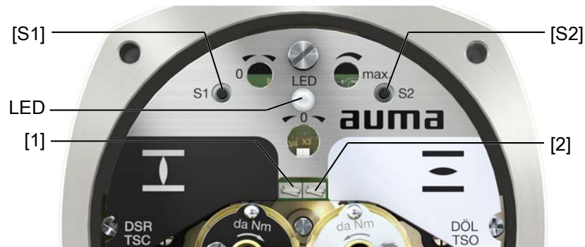
Figure 37: View on control unit when switch compartment is open
