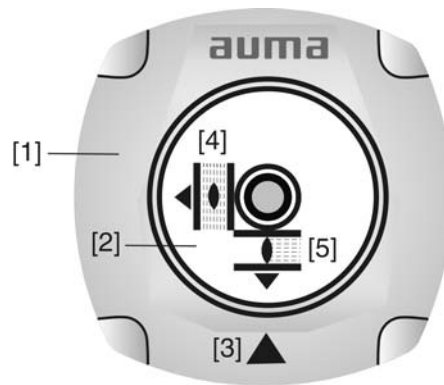
Figure 21: Mechanical position indicator
