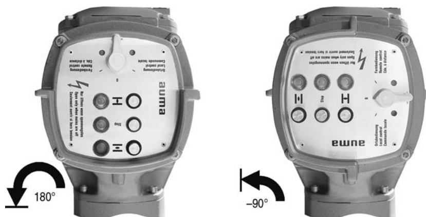
Figure 9: Mounting positions C and D
