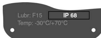
Figure 19: Example: Name plate for enclosure protection IP68
