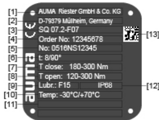
Figure 5: Actuator name plate (example)
