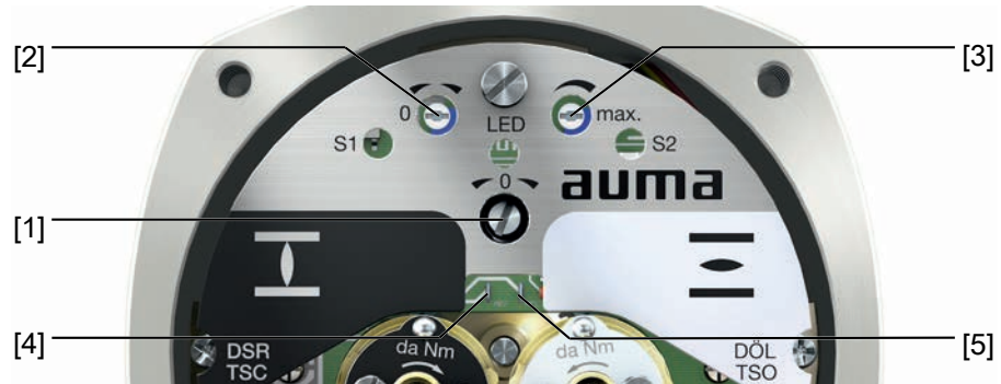
Figure 38: View on control unit when switch compartment is open
