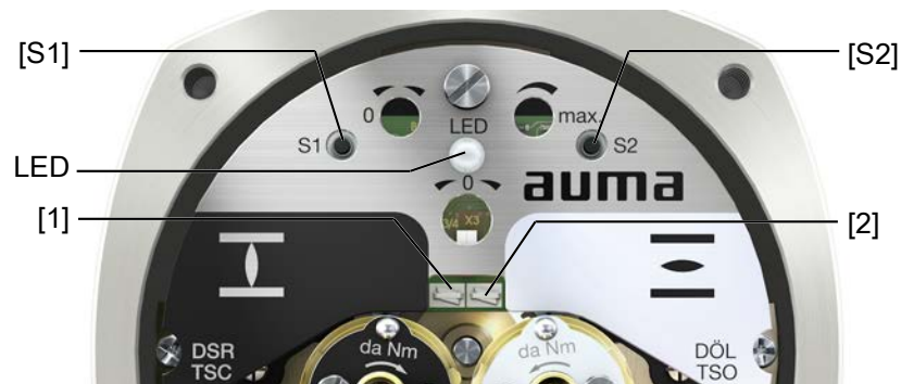
Figure 39: View on control unit when switch compartment is open
