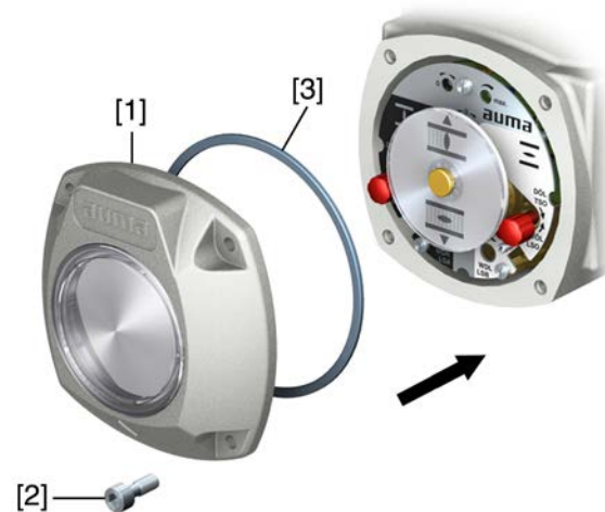
Figure 36: Close switch compartment
