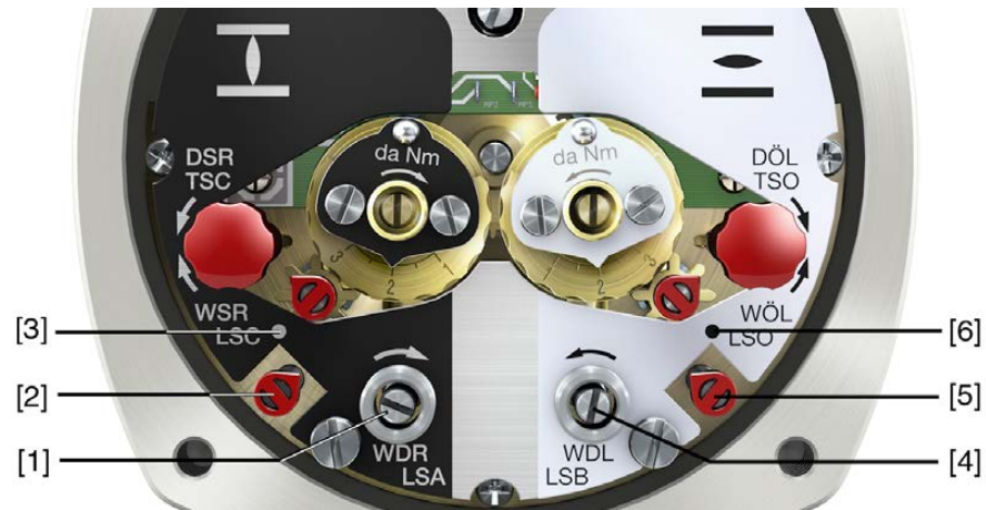
Figure 34: Setting elements for limit switching
