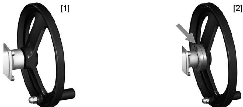
Figure 28: Handwheel without/with overload protection
