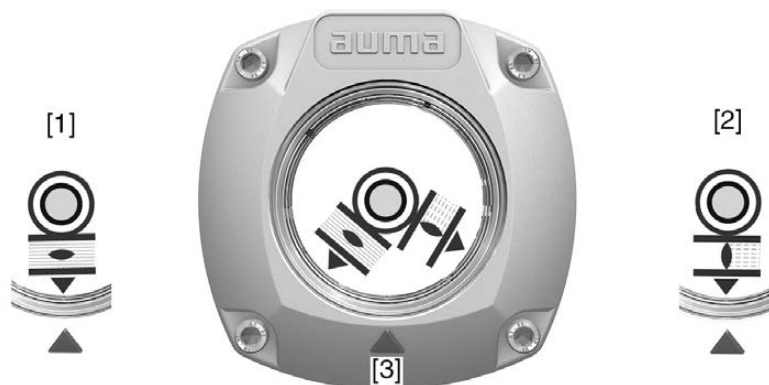
Figure 31: Mechanical position indicator
