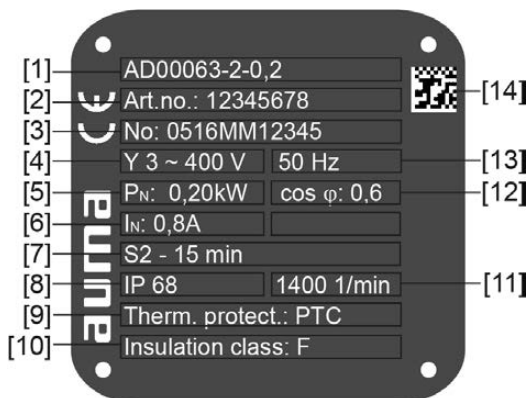
Figure 4: Motor name plate (example)
