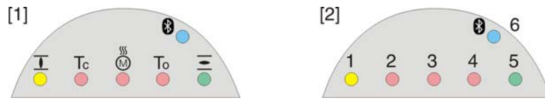
Figure 61: Arrangement and signification of indication lights
