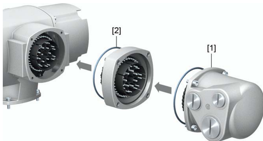
Figure 30: Electrical connection with DS intermediate frame
