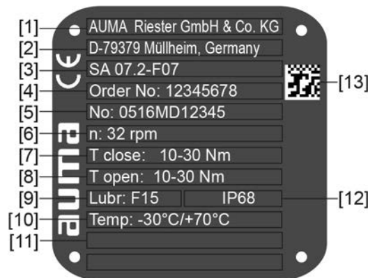
Figure 5: Actuator name plate (example)
